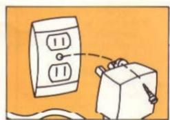
Then, plug the power transformer into a regular wall outlet. It is best to plug the transformer into a wall outlet that is continously "live," not one controlled by a wall switch. You may want to secure the power transformer to the wall outlet as in the sketch above. (Note: Some wall plates may not have a screw location that matches the transformer.)
